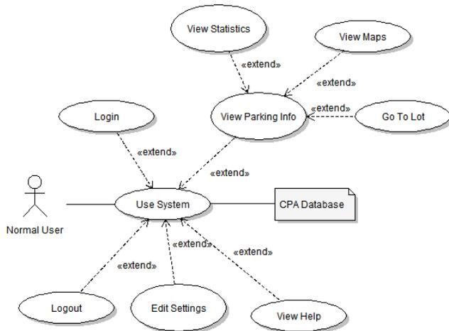
Figure 2. High-level use-case diagram for student CPS parking app project.
